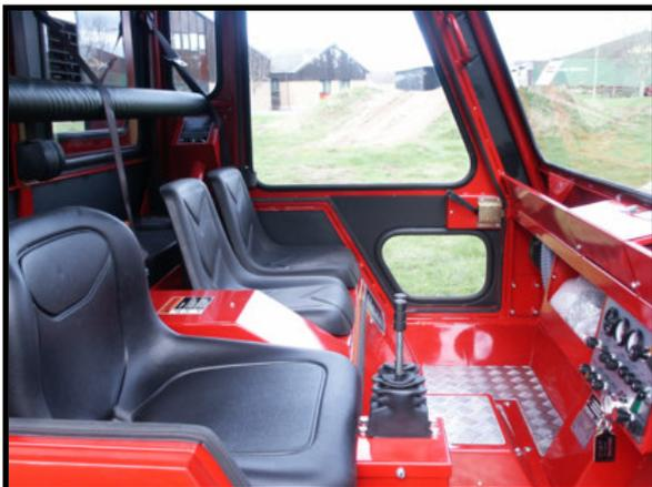
The original PVC canopy has been replaced with a lined and heated hard cab, with lockable doors and opening windows, which is built around a fully certified Roll Over Protective Structure (ROPS). For increased safety and visibility the 3000R comes as standard with four forward facing roof mounted work lamps, a rear directional work lamp, rear position lights and directional indicators.
