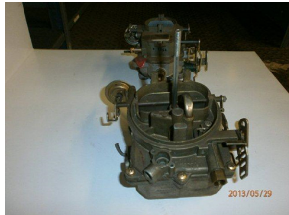
2 Barrel Carburetors, Large Holly and Regular Size Carter
