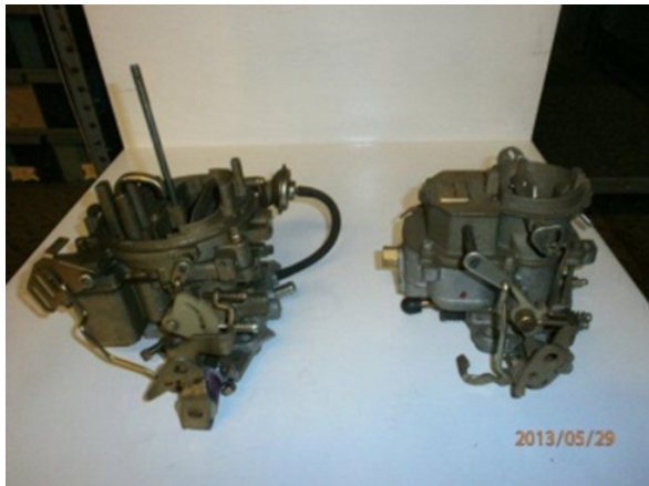
2 Barrel Carburetors, Large Holly and Regular Size Carter
