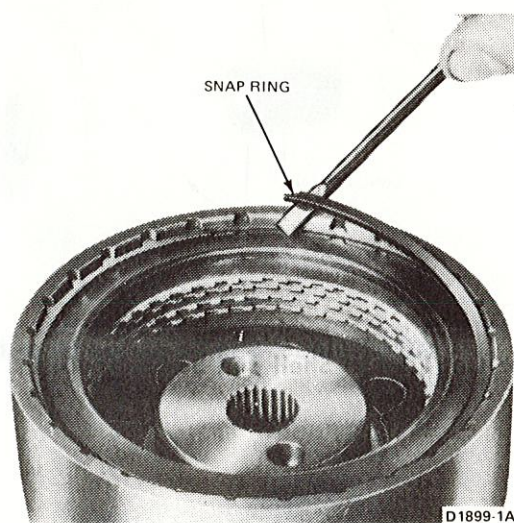
FIG. 44 Removing Forward Clutch Pressure Plate Snap Ring
